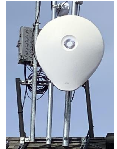
PRM2141 module with 420mm dish and 5GHz backup Approx. > 20 km
